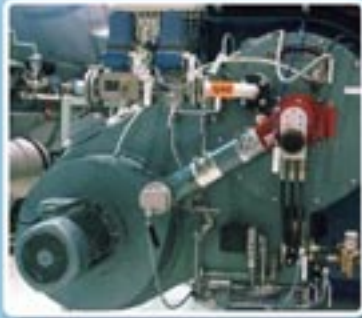
Dual fuel - oil and gas Integrated air fans
