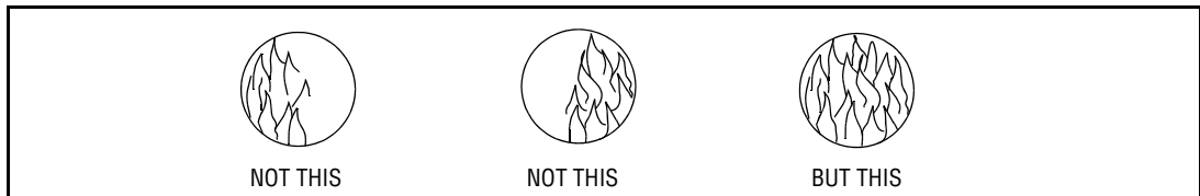
FIGURE 6. FLAME MUST COMPLETELY COVER SIGHT OPENING
